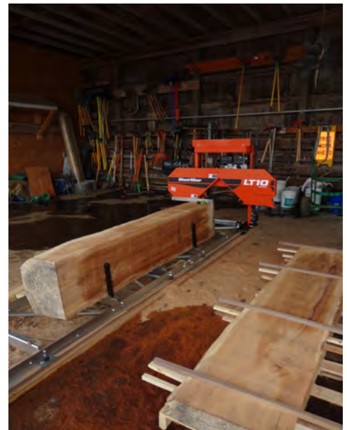
Bandsaw style mill at a local municipality. Photo: Ryan Russell
