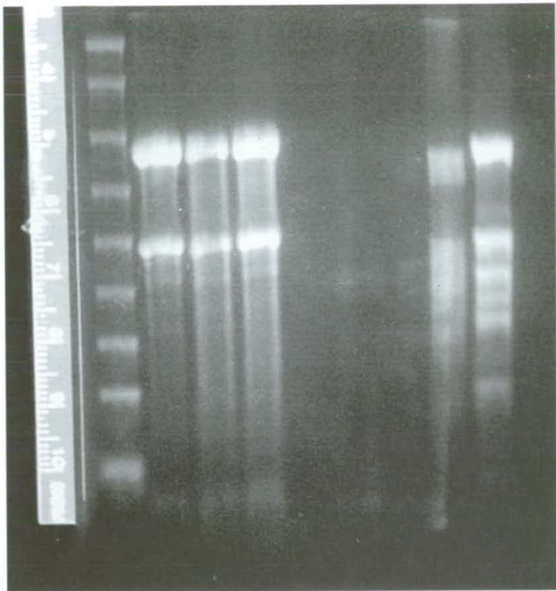
Figure 1. Formaldehyde/denaturing gel of RNA samples from stem shoots (lane 2) and root radicals ( lane 3 & 4). Lane 1 contains an RNA marker used for size identification. (Sigma-Aldrich Company, St. Louis, Mo.)
